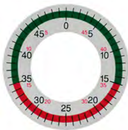
Dial with coloured tolerance fields in red, green or yellow
