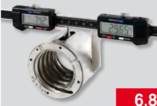
Nutsymmetriemessgerät Digital calipers for slot center distance measuring
