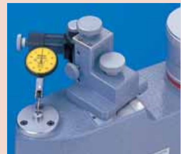
Calibrating test indicator
