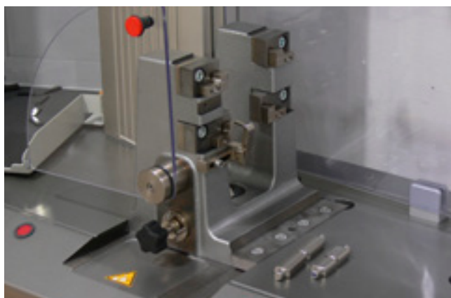
Fig. 1: Charpy fixture with local operator protection, opened
