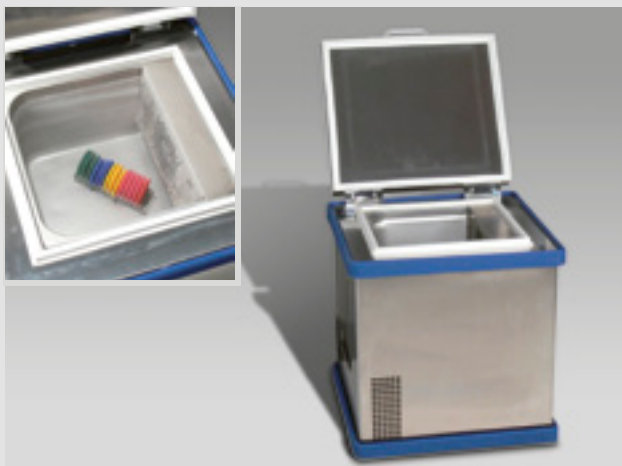
Fig. 3: Thermoregulation box to cool specimens/magazines
