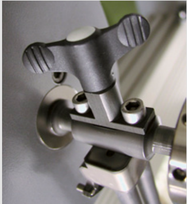
Fig. 1: The pendulum is easily changed by means of a quick release mechanism, eliminating the need for tools.
