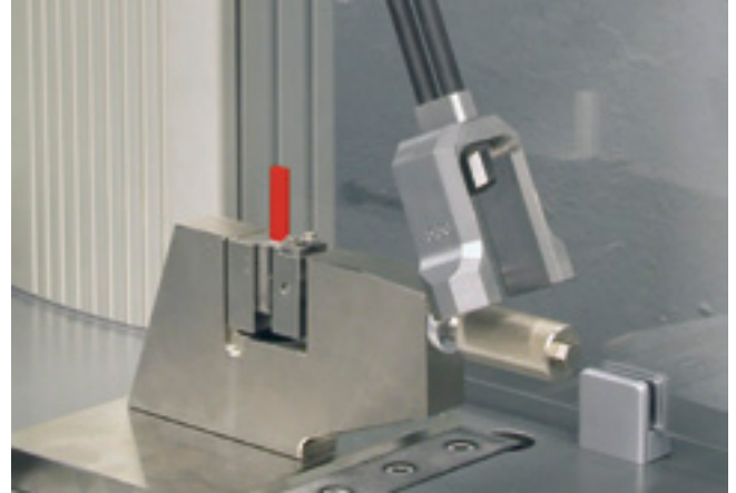
Fig. 1: Test with the manual Izod fixture clamp
