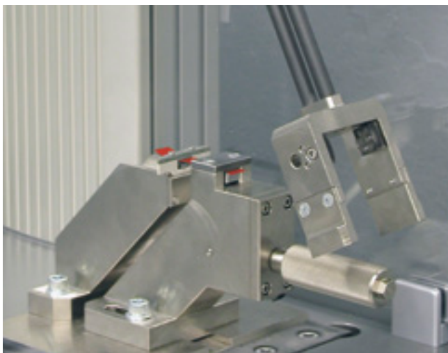
Fig. 3: Fixture for impact tensile tests, Method A
