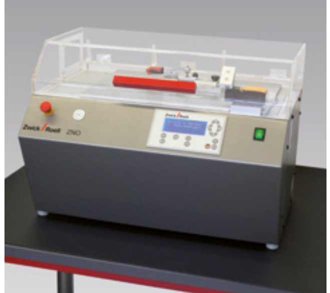
Fig. 1: Notch cutting machine Zwick ZNO with closed safety hood
