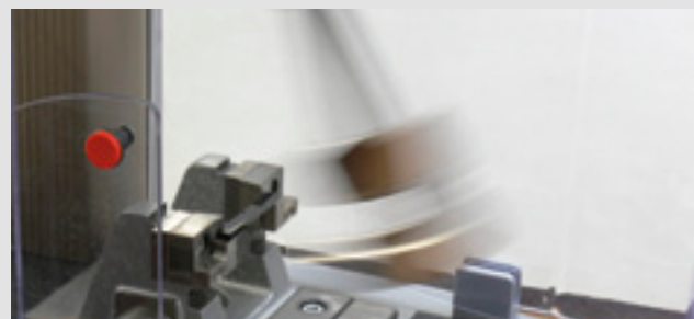
Fig. 3: HIT25P performing a Charpy impact test
