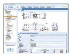
Using the Report Designer within ElcoMaster®, measurements can be quickly displayed on an image or drawing.
