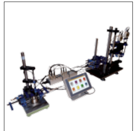
Probes and indicators connection through M-BUS inputs
