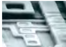
SEM photograph of IC surface after removing upper layer
