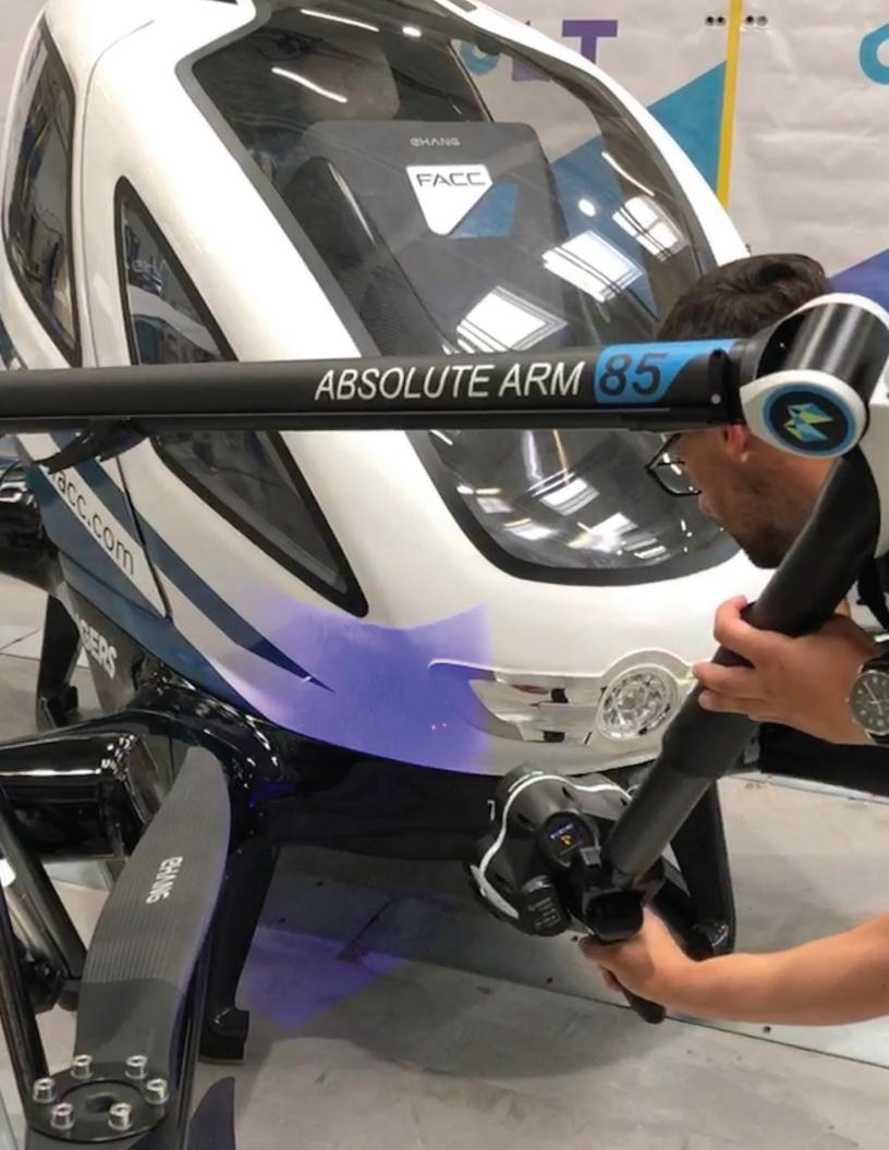
Often, the time needed to scan a part is the most important factor when planning measurement tasks. The part might only be available for measurement for a limited time or restricted to an inconvenient location. That's why Hexagon has created the RS-SQUARED Area Scanner, the world's first structured light scanner mounted on a portable measuring arm.
