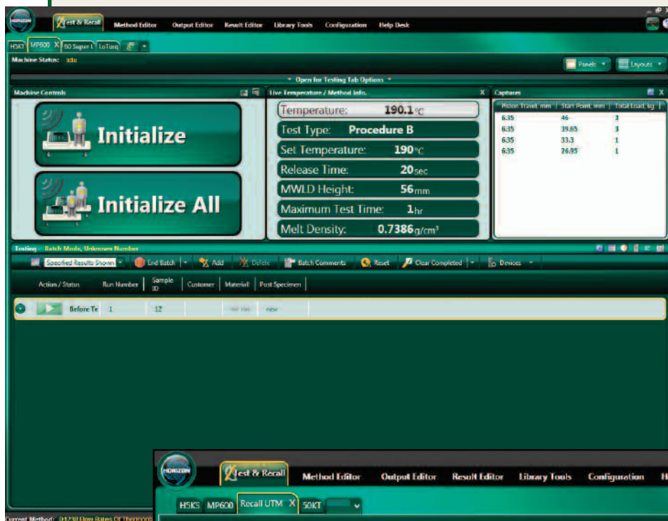
Fig. 5. Test Screen showing the tab labeled for multiple MP600 Melt Indexers. The software is ready to start the tests on multiple MP600 while at the same time controlling the tests being performed on the first tab, which in this example, is an H5kT tensile tester.
