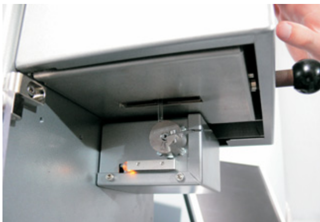
With the automatic extrudate cutter, the extrudate can be cut at precise time intervals
