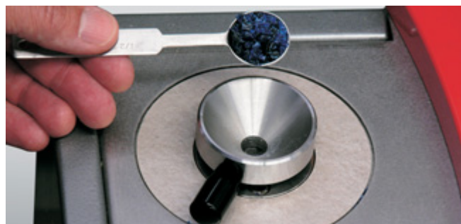
Easy filling of the extrusion barrel with the measuring spoon
