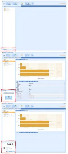
Once the gauge has been connected to ElcoMaster<sup>™</sup> 2.0 (see pages 33 -35), switch on your gauge and click the 'Live Readings' button on the ViewAction Tab
