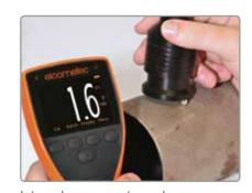
Integral or separate probes measure profiles up to 500µm (20mils) on flat or curved surfaces\*\*
