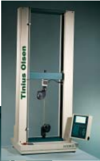
Fig 33. Model H10kS using split bollard grips to test yarn
