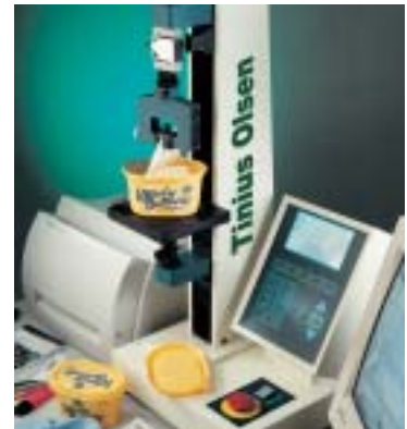
Fig 19. Testing the adhesive peeling forces of foil packaging
