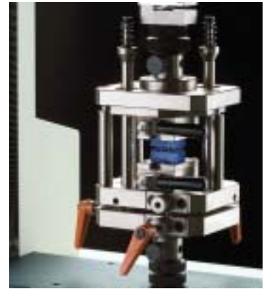
Fig 18. Testing the strength of LEGO blocks with a custom attachment
