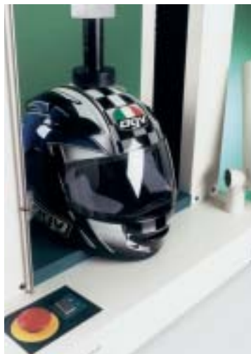
Fig 27. Compression test on crash helmet
