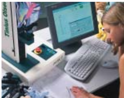
Fig 6. Model H1kT being used to test material and stitching on stuffed toy
