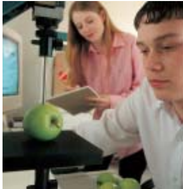
Fig 10. Testing the ripeness of apples using a set of Magnus Taylor probes
