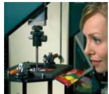
Fig 20. Testing the puncture and bursting strength of packaging material
