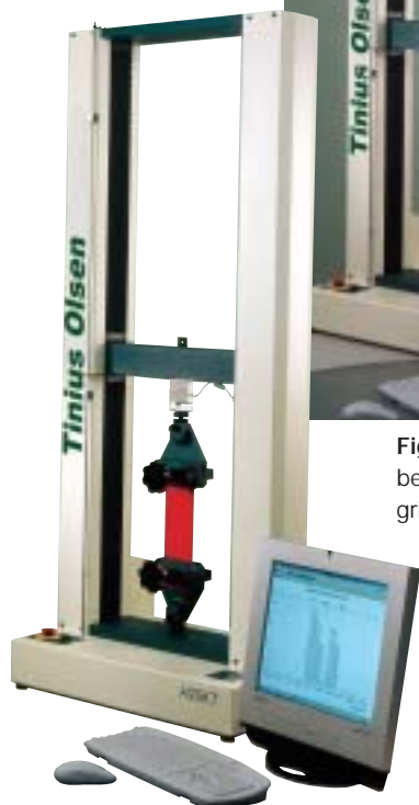
Fig 36. Model H25kT using model HT40 grips to test fabrics
