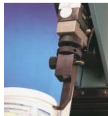
Fig 21. Determining the force to remove the lid from a plastic package
