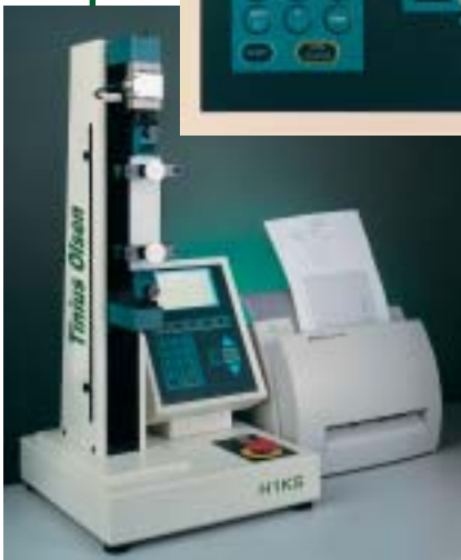
Fig 3. Model H1kS testing paper strips; shown with HT50 tensile grips
