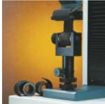
Fig 13. Checking the peeling strength of the outer layer of rubber hose, using a combination of standard and custom grips
