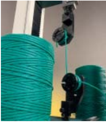
Fig 22. Yarn being tested with split bollard grips
