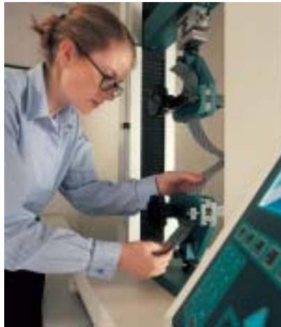
Fig 38. Machine being used to determine the strength of a geotextile
