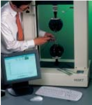
Fig 23. Dumbbell sample of sheet metal being tested with HT21 grips
