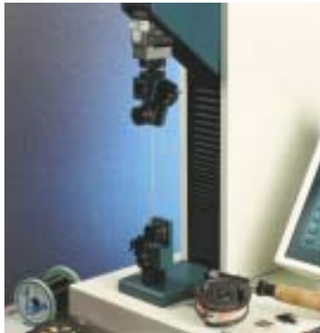
Fig 12. Testing the strength of fishing line using single bollard grips, HT33
