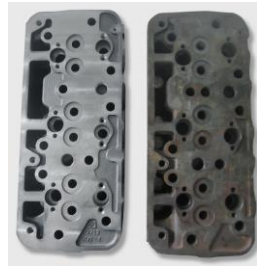
Reverse Engineering of a historical cylinder head
