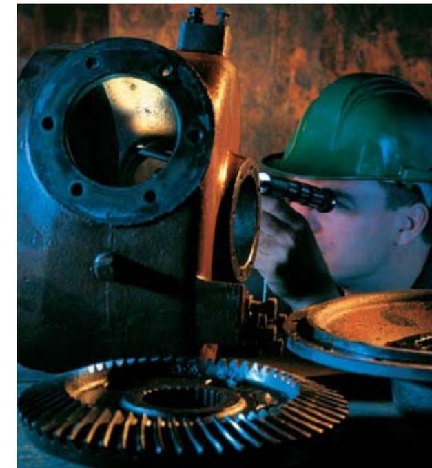
Rigid Borescope inspection of power take-off transmission
