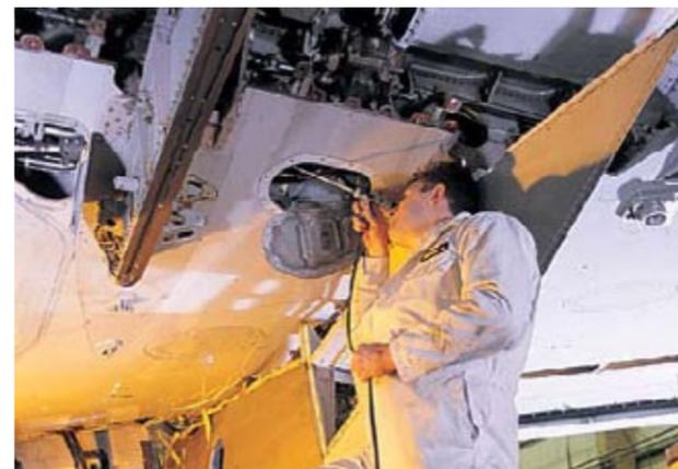
Inspection of hard-to-reach area of airframe structure
