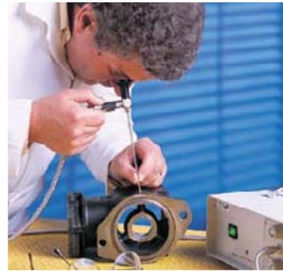
Inspecting air-brake compressor after machining
