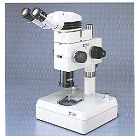
COX Coaxial vertical illuminator mounted on the RZT Stand model
