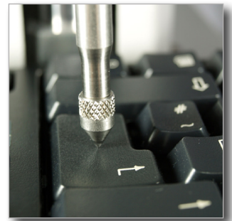
Keypad compression test
