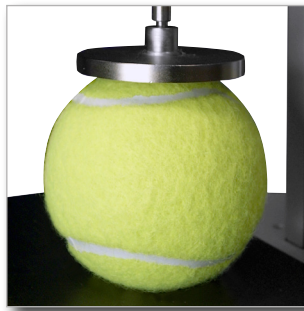
Tennis ball compression test
