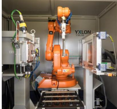
**Automated X-ray systems with robots for the for the inspection of cast parts**
