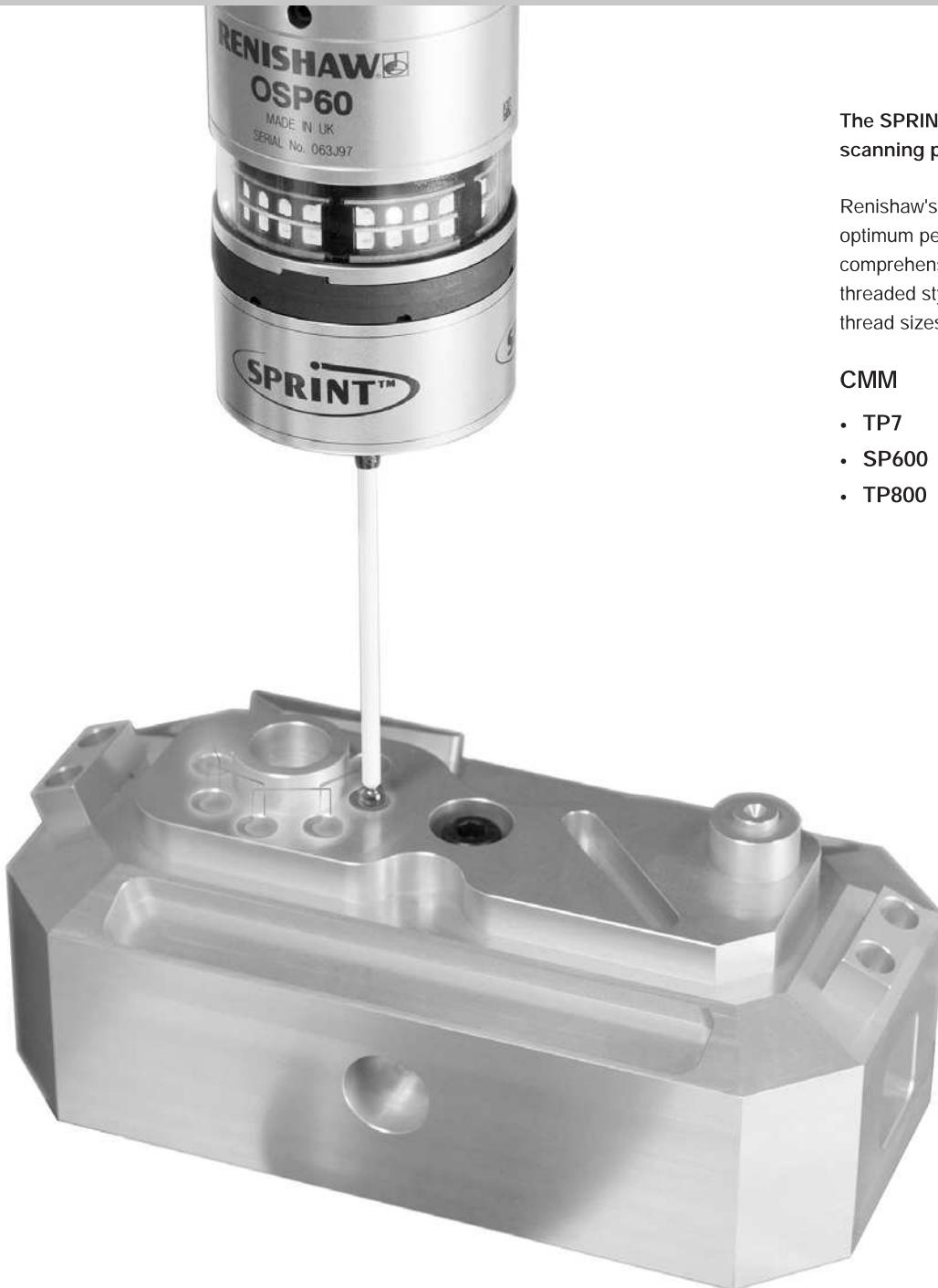
The SPRINT OSP60 is a high-speed optical 3D scanning probe for machining centres
