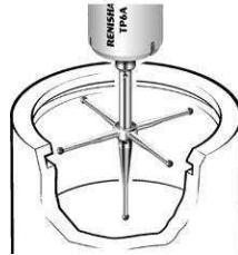
These stylus clusters provide you with multiple-tip probing of complex features and bores. Four or five ruby ball systems are mounted rigidly on a stainless steel centre. Three standard sizes are offered – alternatively, you can create custom-made star styli using a 5-way stylus centre and any of the genuine Renishaw stylus range.
