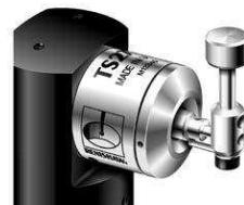
Typically, these are fitted with a square tip and can have threaded or plain shaft attachments. The tip faces are ground to ensure high squareness and parallelism. The TS27R tool setting probe for machining centres can also be fitted with a tungsten carbide disc stylus.
