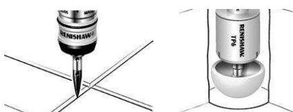
Pointer styli are designed for the inspection of thread forms, specific points and scribed lines (to lower accuracy). The use of a radius end pointer stylus allows more accurate datuming and probing of features as detailed above and can also be used to inspect the location of very small holes.
