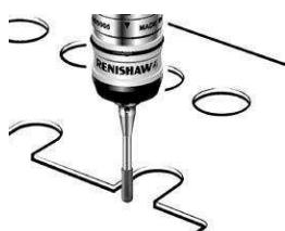
These are used for probing holes in thin sheet material. In addition, various threaded features can be probed and the centres of tapped holes located. Ball-ended cylinder styli allow full datuming and probing in X, Y and Z directions, thus allowing surface inspection to be performed.
