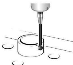
These are the simplest form of stylus, incorporating highly spherical industrial ruby balls and a choice of stem material.
